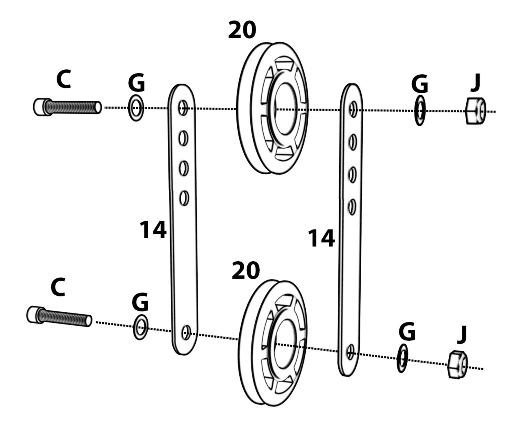
Assemble the connector pulley as pictured in the diagram above and place between the cables in the next step
