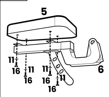
Assemble and secure the seat cushion to the adjustable frame.
