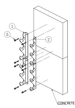
NO. DESCRIPTION **O'TY** 1 Gun Rack (Left Side) 2 2 2 Gun Rack (Right Side) 3 8 Wood Screws (M8\*60mm) 8 4 Washers (8mm Diameter) 5 8 **Concrete Screws (8mm)**
