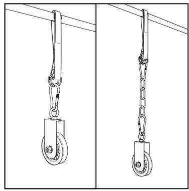
**Step 2:** Attach the pulley to the hanging strap. If the mounting beam is high up, the chain extender is provided to set the pulley at a manageable height: attach the chain to the hanging strap and the pulley to the opposite end of the chain.
