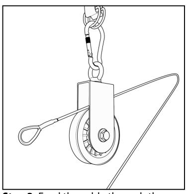
**Step 3:** Feed the cable through the pulley.
