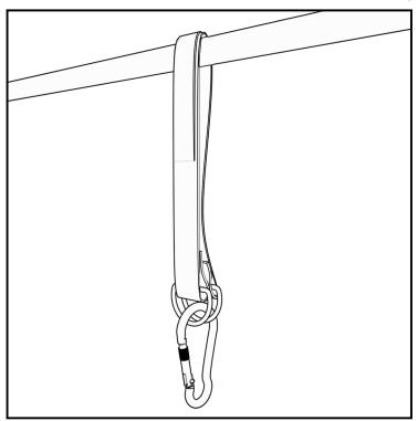
**Step 1:** Attach the hanging strap to a secure raised mounting beam.
