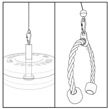
**Step 4:** Attach the plate stacker to one end of the cable and attach the tricep rope to the other end of the cable.
